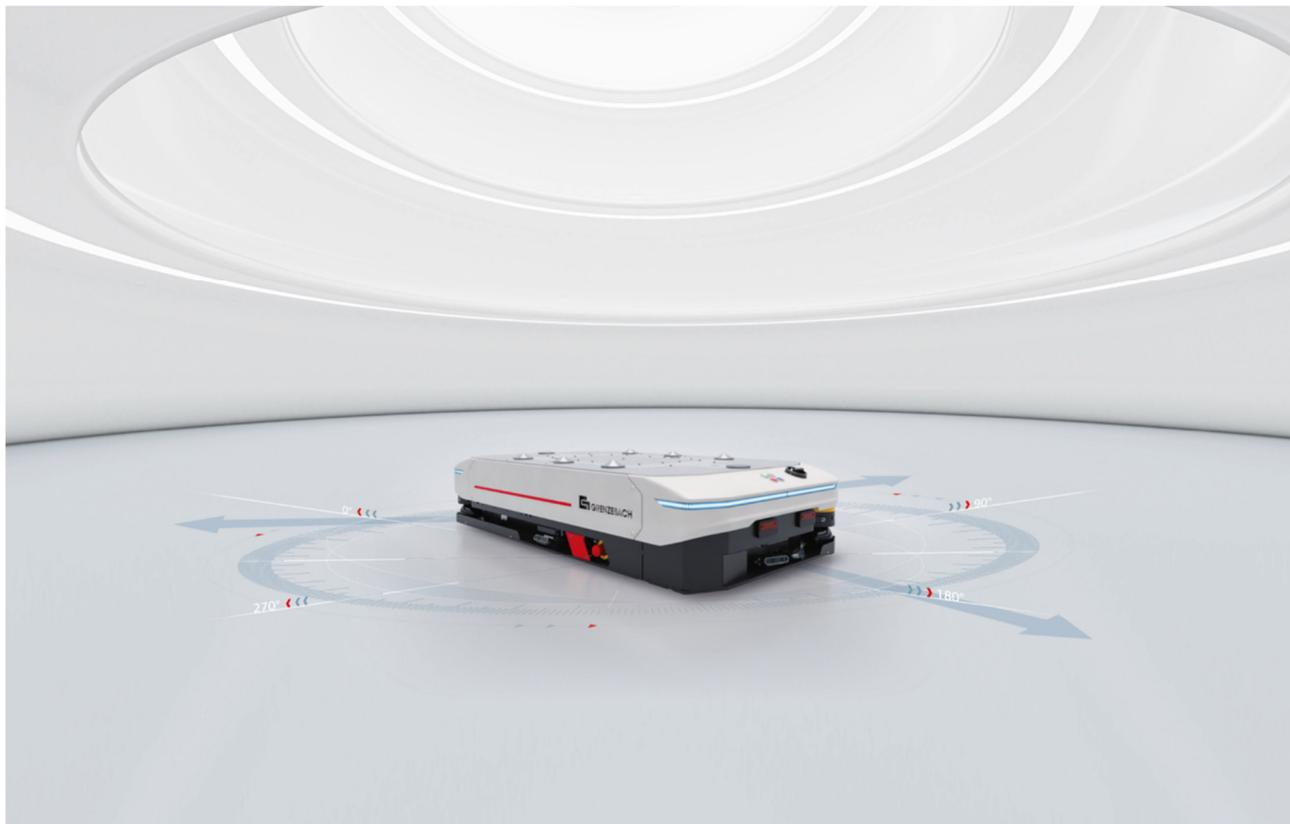
*360° Head Start: Thanks to its omnidirectional drive and smart sensors, the Automated Guided Vehicle OL1200S from Grenzbach allows easier, quicker, and safer transportation, particularly of long goods carriers.*
