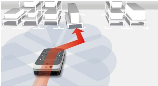
Autonomous Load Carrier Detection
